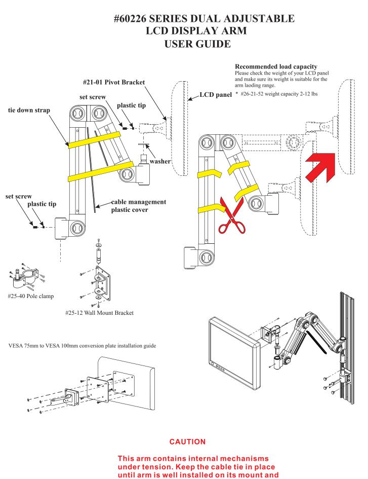
until arm is well installed on its mount a the device is well attached to the arm to avoid serious injury.
